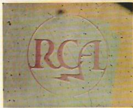
A snapshot records RCA's first successful use of color in a liquid-crystal display, 1965.
